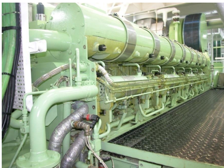
The common-rail 8L32/44CR engine aboard the Playa de Azkorri
