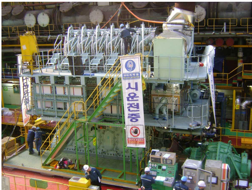
The MAN B&W 6S50ME-C7 engine pictured on the testbed at HHI-EMD in January 2010
