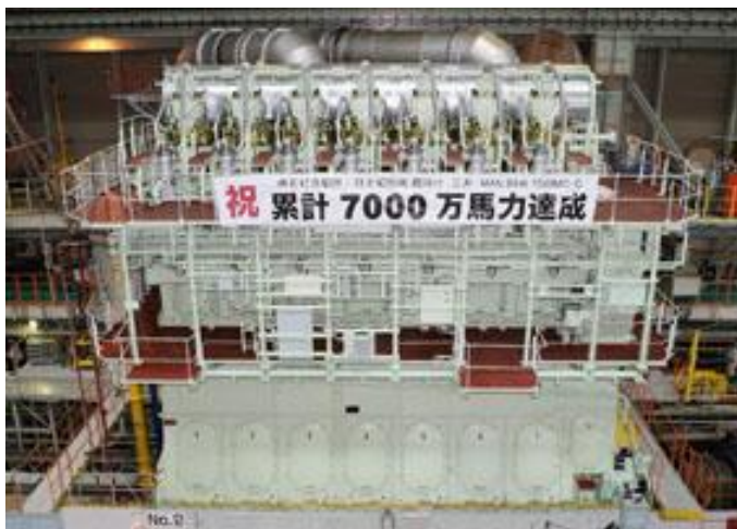
The MAN B&W 7S80MC-C7 engine pictured at production in Tamano
