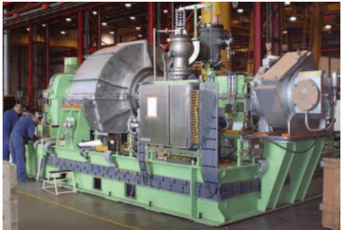
Fig. 4: The complete turbine generating set. The unit for an MAN B&W Diesel 12K98ME/MC engine measures only 10 m by 3.5 m.
