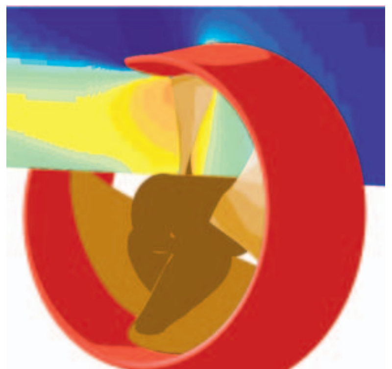
Fig. 4. The 3D slice-cut model of nozzle, propeller blades and hub for the AHT design. This model clearly shows how smoothly the higher pressure increases across the whole blade width.
