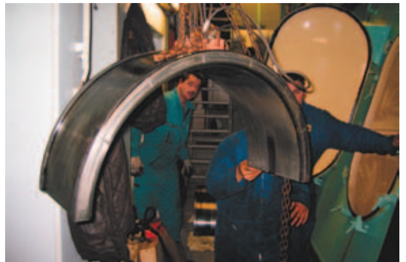
Upper bearing shell removed to allow further inspection.
