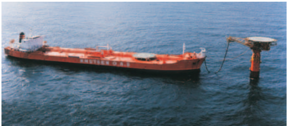
'Anna Knutsen' vessel data: delivered in December 1986 from Moss Rosenberg Verft / Moss Fredrikstad Verft, Norway, as yard no. 443. Deadweight: 123,819 tons. Main engines: 2 x MAN B&W 4L70MCE (9,760 BHP @ 95 rpm). Two main engine driven alternators (PTO gears). Propellers: 2 x CPP, diameter 6.1 m. Side thrusters/rudders: Two tunnel thrusters and two Becker Rudders. Two electrohydraulic steering gears.
