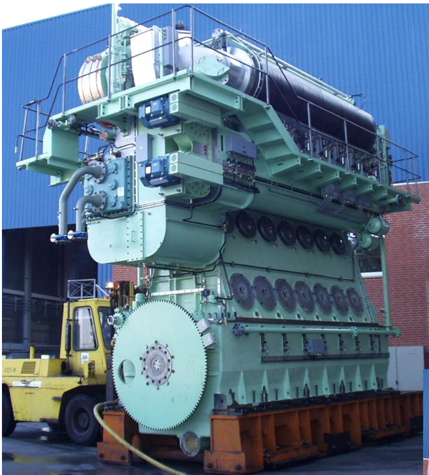
One of the two 7S35MC engines ready to ship to Vietnam
