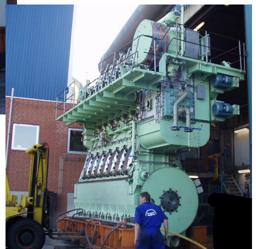
One of the two 7S35MC engines ready to ship to Vietnam
