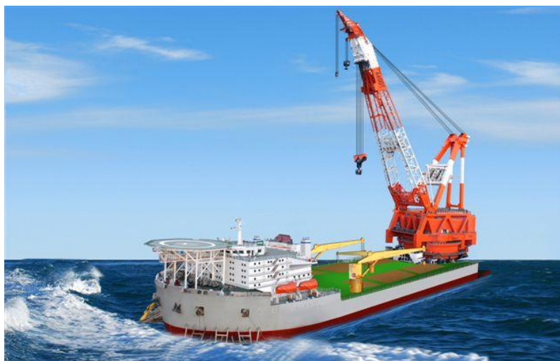
Graphic impression of ZPMC's new large DLV 4400 floating crane with a lifting capacity of 4,400 ton
