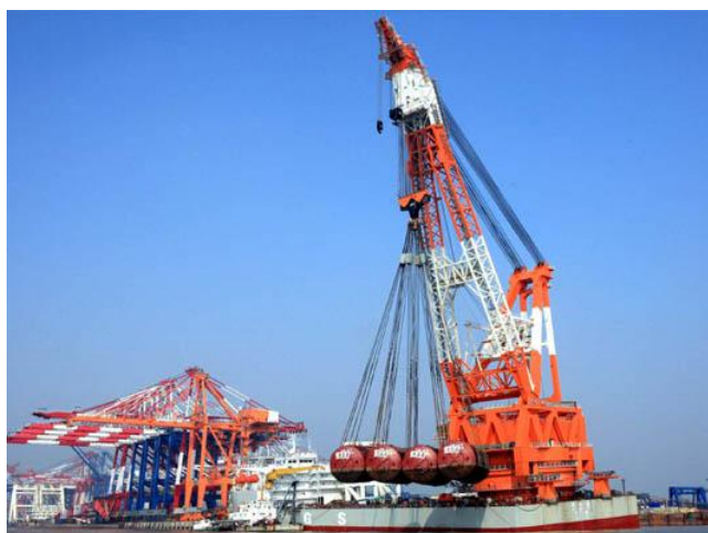
Two photos: The DLV4000 floating crane performing its trial lifting test of 4,000 ton at sea and at quayside
