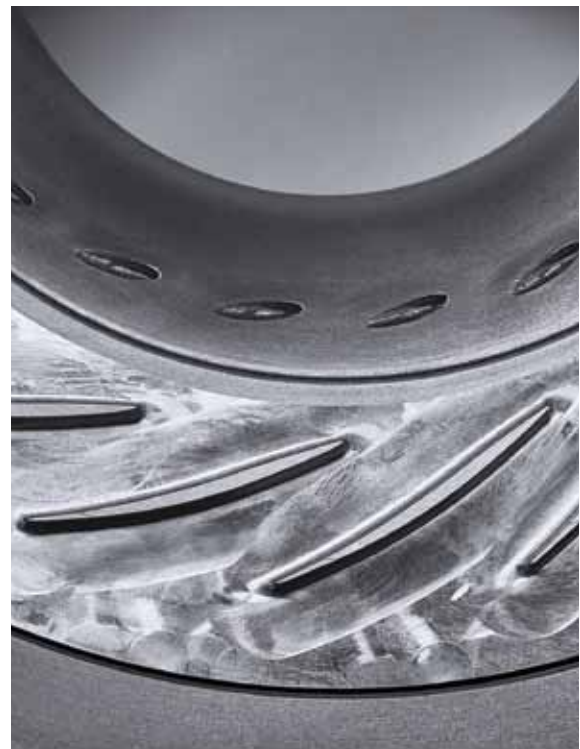
Insert piece with jet assist bores, diffuser
